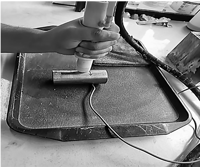
FIGURE 7 Electropolishing the specimen in the circumferential direction.
