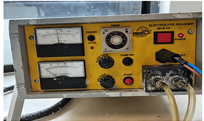
FIGURE 6 Proto electropolisher for removal of the surface layer.
