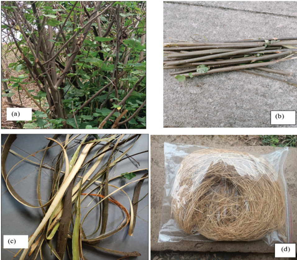
Figure 1. Macroscopic image of (a) Dombeya buettneri plant, (b) stem, (c) bark, and (d) fibers.
